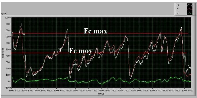
Figure 9 : Experimental PDC forces during rock cutting
