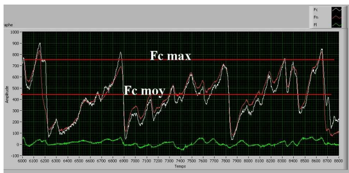
Figure 9 : Experimental PDC forces during rock cutting
