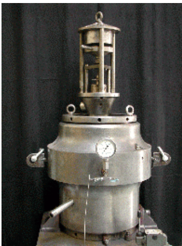
Figure 8 : confinement single cutter test stand
