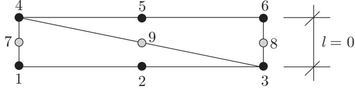
Figure 3: Kinematically admissible velocity discontinuity comprised of two quadratic elements of thickness  $l$  set to zero.
