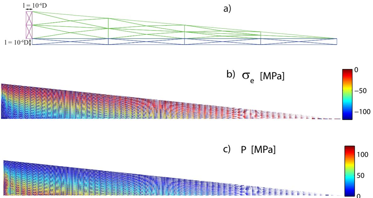
Figure 5: The type of mesh over the wedge, including the collapsed elements for the interfaces, a). The two invariants of the stress-like results, the in-plane mean stress  $P$  b), and the equivalent stress  $\sigma_e$  for  $\alpha = 3^\circ$ , c), corresponding to sub-critical slope conditions. Units: MPa.
