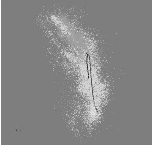
Fig.1: Plan view of the locations of the generated events at Soutz after the hydraulic stimulation of GPK2 borehole (top trace), GPK3 borehole, and GPK4 borehole (bottom trace)
