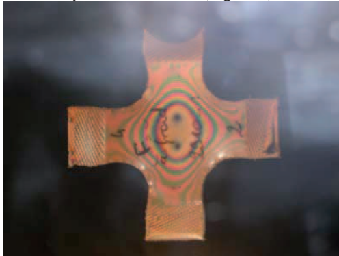
Fig. 8. Birefringence pattern observed on a PET specimen, equi-stretched, at a temperature of 100 °C and arms velocity of 0.1 \text{ mm}\cdot\text{s}^{-1} , with an equivalent draw ratio of 1.9. The specimen has been ambient air cooled.
