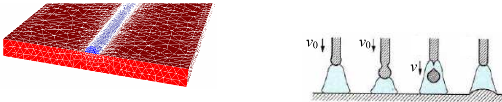
Figure 2. On the left, the meshes of the plate (in red) and of the box for weld bead formation (in blue). On the right, different steps of the weld joint formation.
