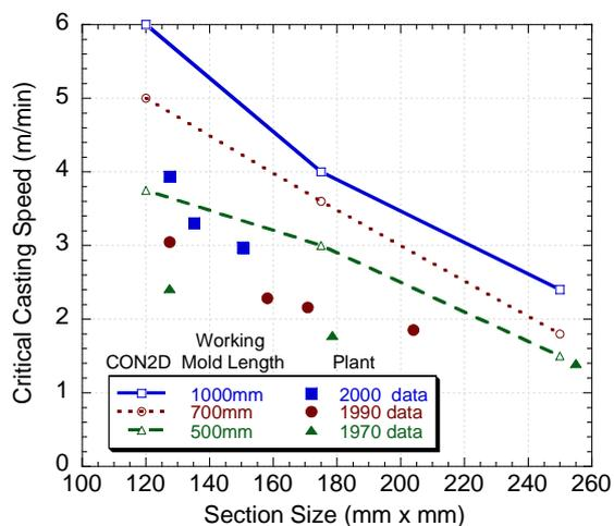
Figure 27.14. Comparison of critical casting speeds, based on hot-tearing criterion, and typical plant practice.<sup>72</sup> (After Li, C. and B.G. Thomas, Thermo-mechanical Finite Element Model of Shell Behavior in Continuous Casting of Steel, Modeling of Casting, Welding and Advanced Solidification Process X, San Destin, FL, May 25-30, 2003, TMS, 2003.)
