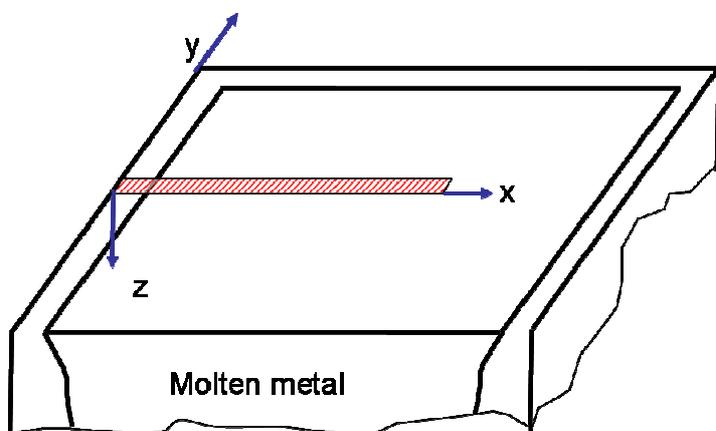
Figure 27.2. One-dimensional slice-domain for modeling solidifying plate.
