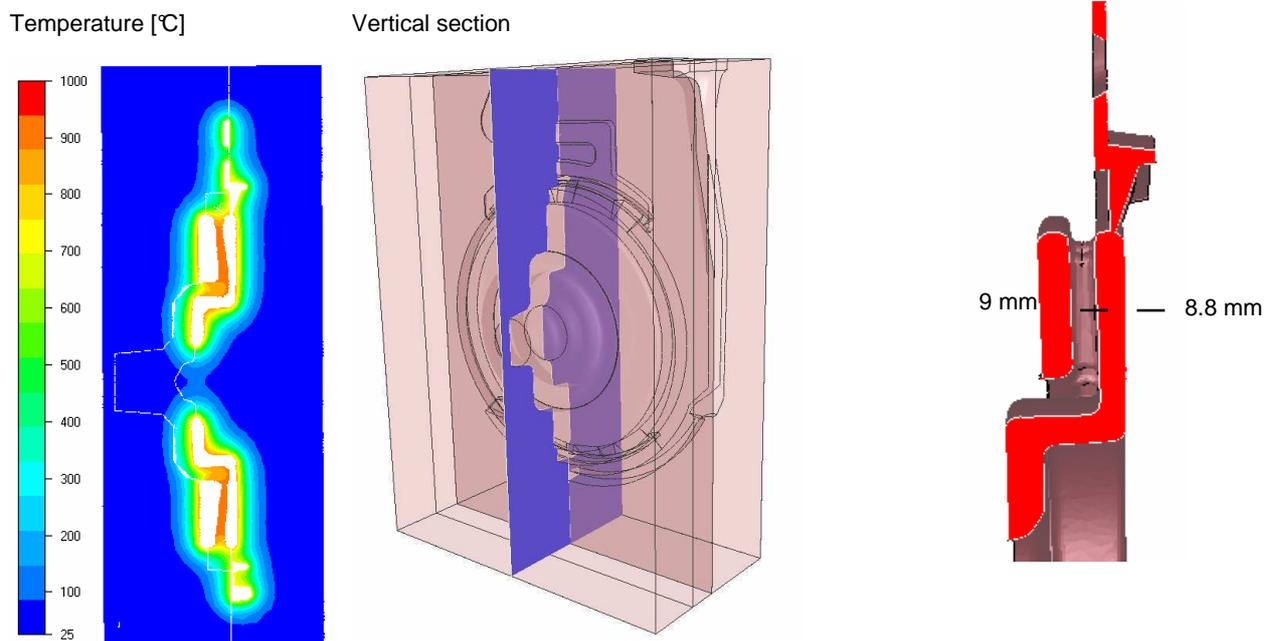
Figure 27.7. Deformation of core blades in a radial section, after a few seconds of cooling. On the left, displacements have been magnified by a factor 100. The temperature distribution is superimposed. On the right, the difference in thickness between the two braking tracks is shown.
