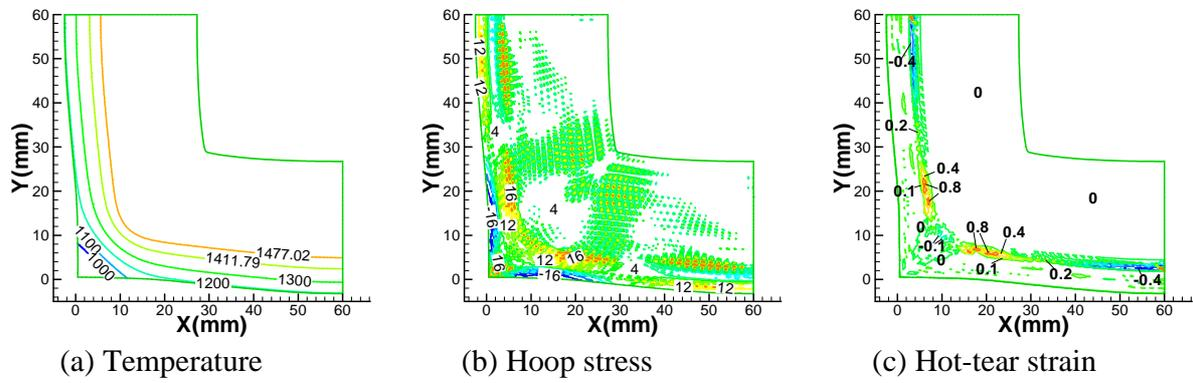
Figure 27.11. Distorted contours at 200 mm below mold exit.
