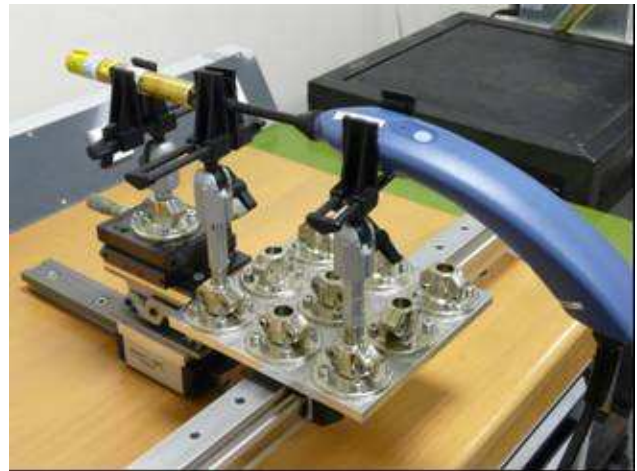
Fig. 10. Photo of the LNE test bench to qualify the refrigerant leak detectors according to the standard NF EN 14624
