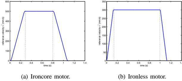
Fig. 2. Reference velocity profiles in  $mm/s$ .
