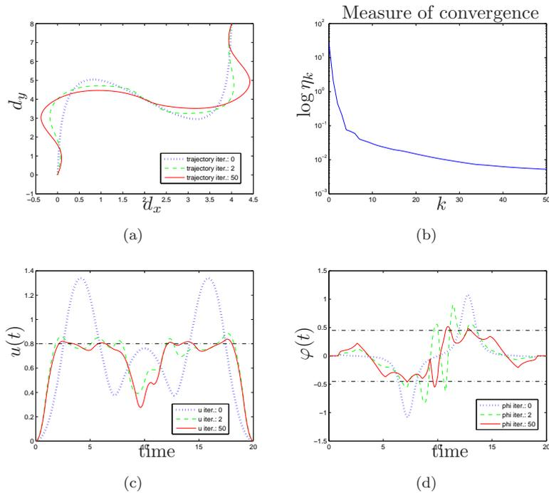
Figure 1: Initial reference trajectory, 2<sup>nd</sup> and 50<sup>th</sup> iteration. (a) Flat output  $y = (d_x, d_y)$ ; (b) Measure of convergence  $\eta_k$ ; (c) Input  $u(t)$ ; and, (d) Input  $\varphi(t)$ .
