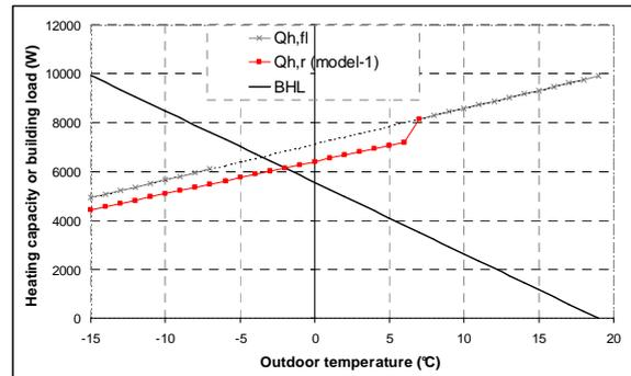
Figure 3 – Defrost effect on full load heating capacity
