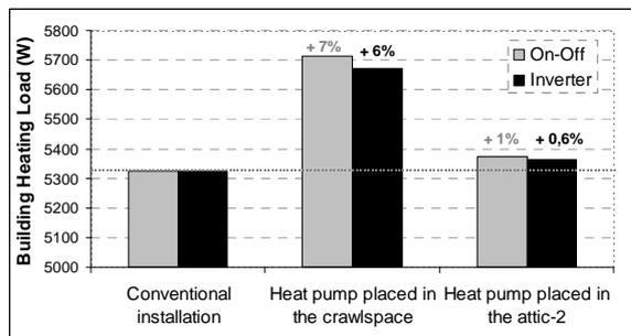
Figure 8 – Building heating load according to the configuration
