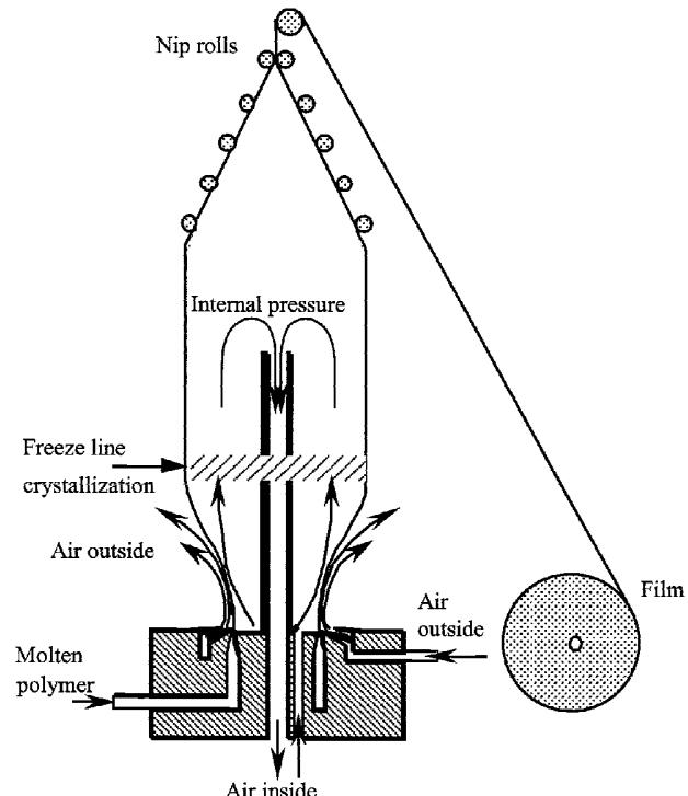
Figure 1 – Schematic diagram of the film blowing process.
