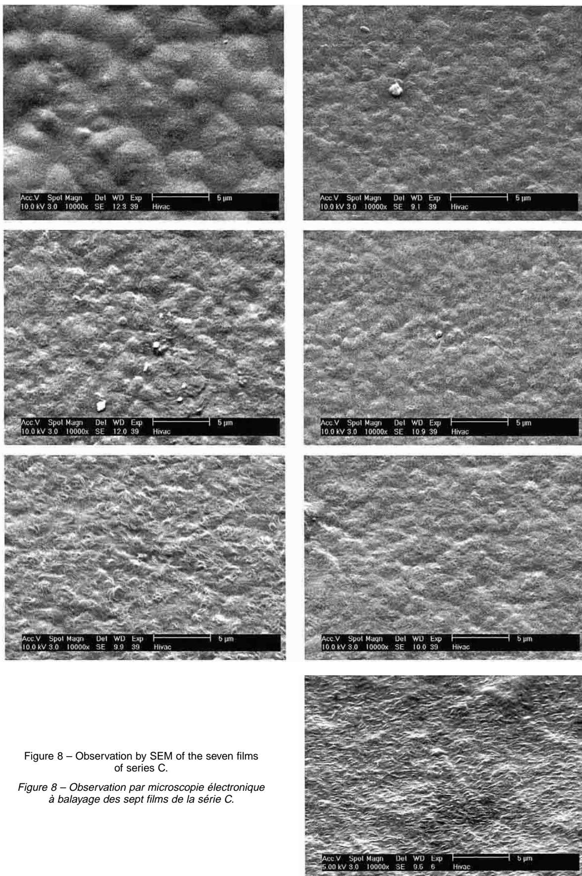
Figure 8 – Observation by SEM of the seven films of series C.
