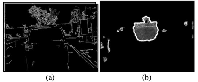
Figure 6. Illustration of the verification using lack of contours property. (a) is the sum of contours in frame  $n-1$  and  $n$ . Gray edges belong to frame  $n-1$  while white ones are from frame  $n$ . (b) As a result of the subtraction, only the connected component surrounded by white contours will be validated for further stages.
