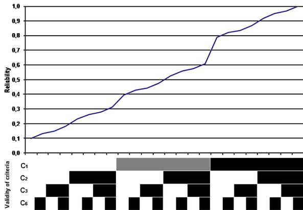
Fig. 5. Evolution of the reliability measure of the sensor depending on the validity of each criterion. The curve shape is conditioned by  $C_1$ ,  $C_2$ ,  $C_3$  and  $C_6$  values. When all criteria are validated, confidence in the evaluation of the belief function by the source is high. Practically,  $m_{rel}$  is close to 1 and conversely close to 0 when dealing with an unreliable sensor.
