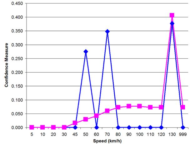
Fig. 6. Comparison between Lauffenburger method (◆) and ours (■). The situation corresponds to a reliable sensor, meaning that all criteria of  $C_{rel}$  are validated on a highway. The speed limit stored in the database is 130 km/h.
