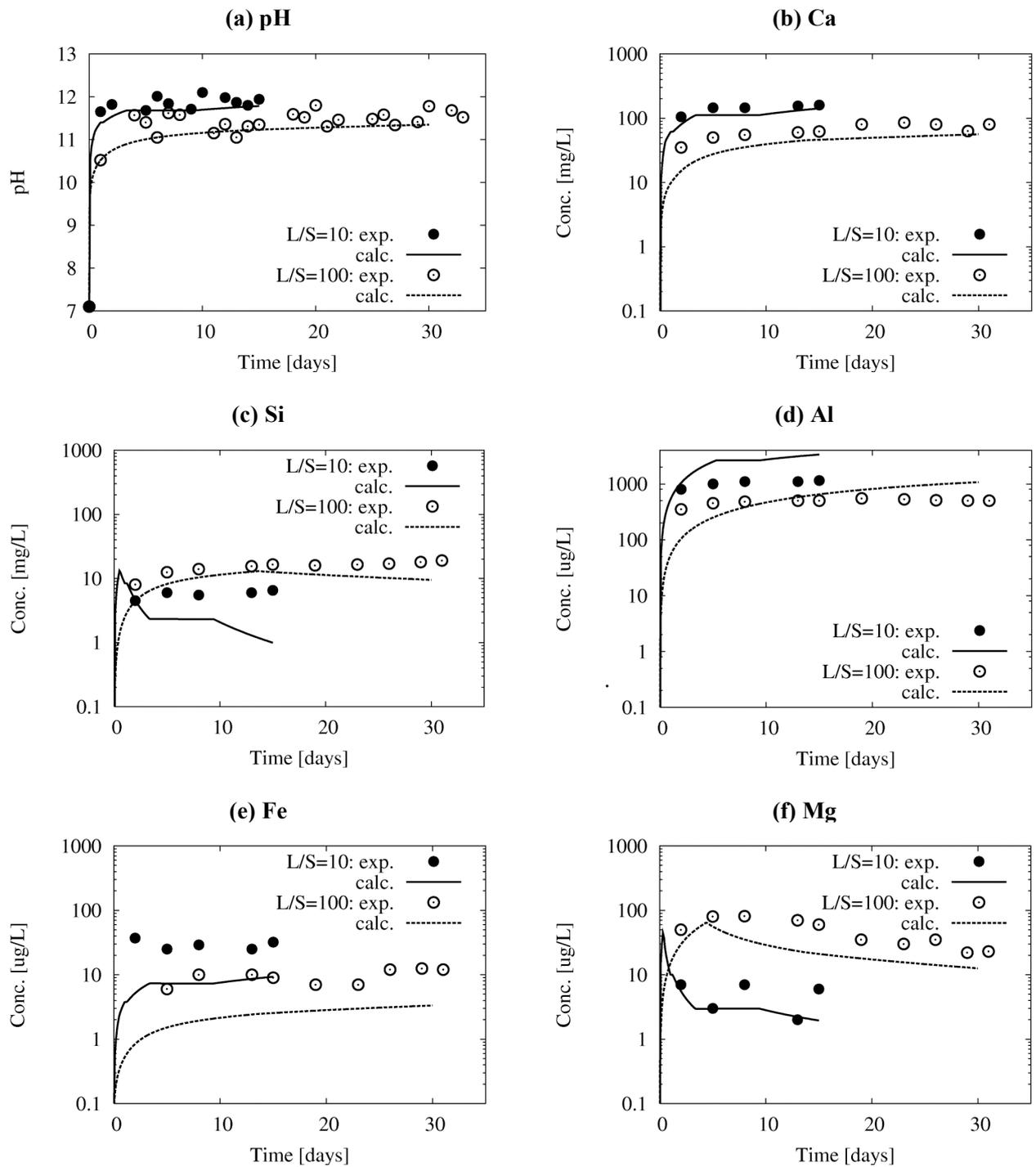
Fig. 1. Experimental (exp.) and calculated (calc.) evolution with time of pH (a) and concentration of the main BOF steel slag elements in the batch leachates (b-f).
