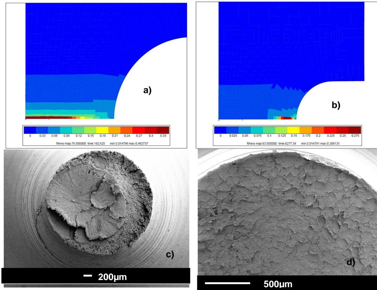
Figure 7: Comparison between damage contour map and fracture surfaces: a) and c) NT0.8, maximum porosity as well as ductile surface located in the centre; b) and d) NT0.45, maximum porosity and ductile surface next to the notch root.
