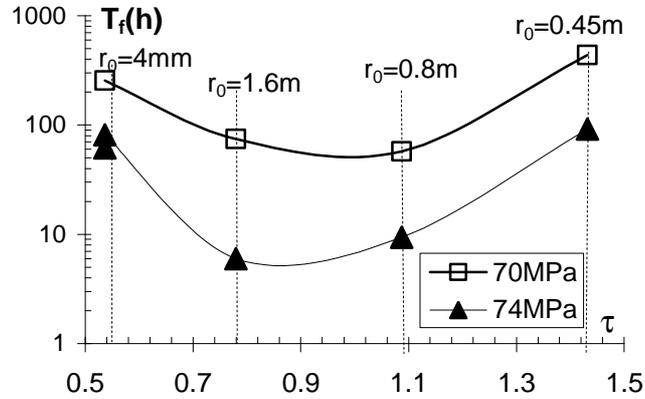
Figure 2: Time to failure versus stress triaxiality: higher creep lifetime for  $r_0 = 0.45\text{mm}$
