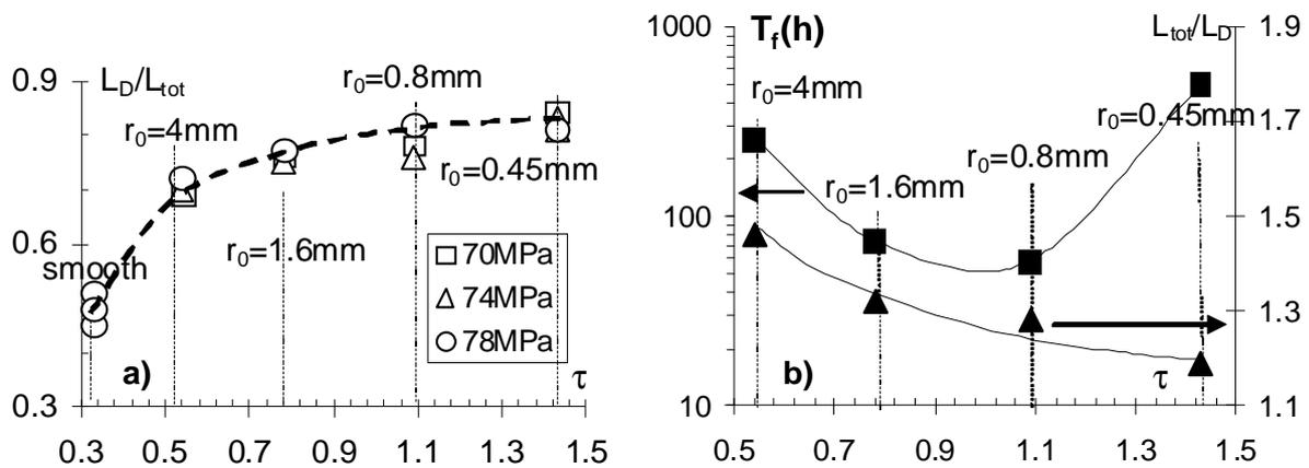
Figure 5: Ductile length fraction vs. stress triaxiality ratio  $\tau$ . a) for three applied net stresses; b) for 70MPa where the time to failure was superimposed.
