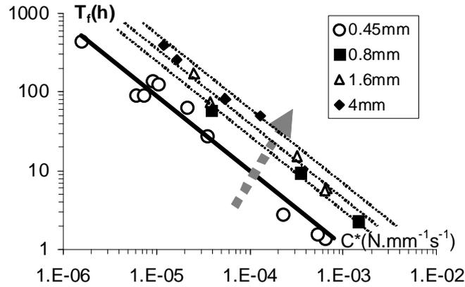
Figure 6: Time to failure vs.  $C^*$  master curve for PA6 at room temperature.
