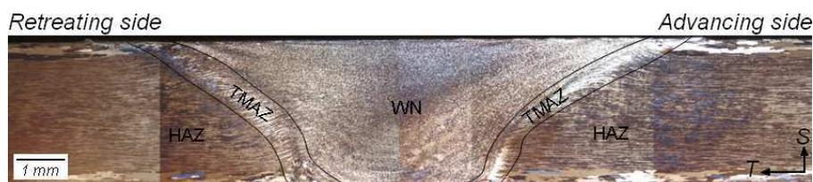
Fig. 4: Light optical micrograph of a JLR-free weld
