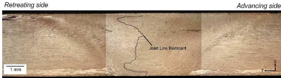
**Fig. 5:** Light optical micrograph of a JLR-bearing weld (JLR line redrawn artificially to highlight its morphology)
