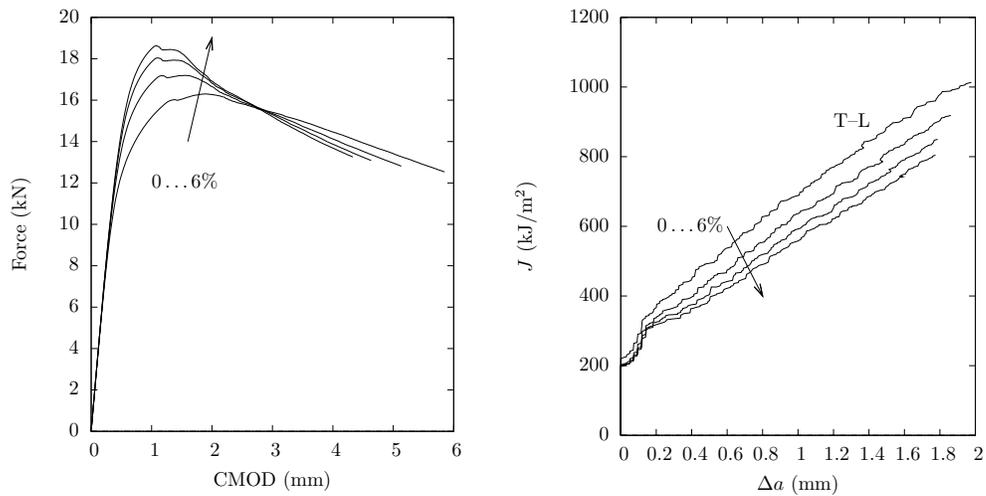
Figure 6: FE simulation of CT tests carried out in the T-L configuration for various prestrain levels. Load-CMOD curves and  $J$ - $\Delta a$  curves.
