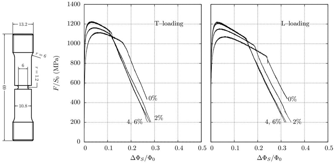
Figure 2: Test results for notched bars ( $r = 1.2$  mm) tested along the T and L directions for the various prestrain levels. ( $F$ : force,  $S_0$ : initial minimal cross-section,  $\Phi_0$ : initial minimal diameter,  $\Delta\Phi_S$ : minimal diameter variation along the S direction).
