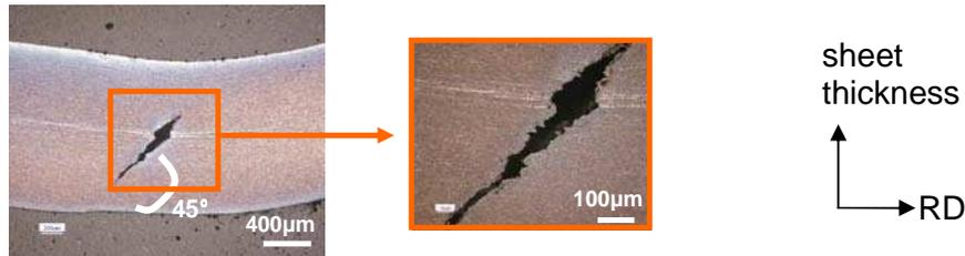
**Fig. 8:** Stretch bent specimen; the test was interrupted after internal cracking. Optical micrographs, LePera etching
