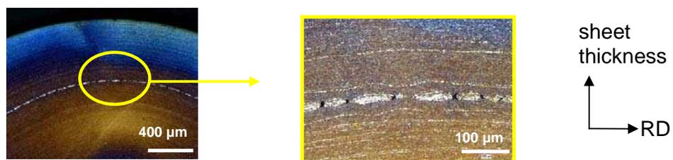
Fig. 6: Local necking around the central segregation band, optical micrographs, LePera etching
