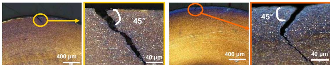
Fig. 5: V-bending specimens. Optical micrographs, LePera etching
