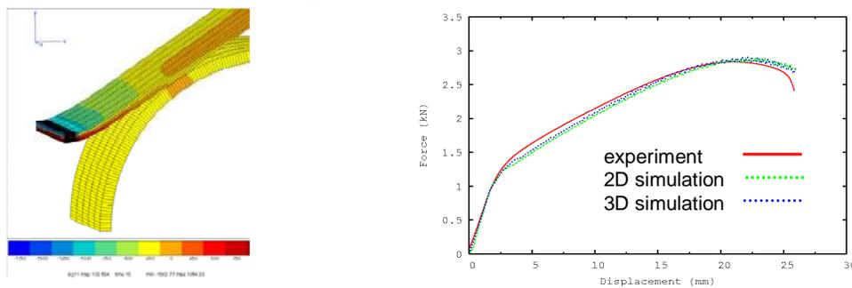
Fig. 13: Left:  $\sigma_{11}$  map of the 3D V-bending test ( $\sigma_{11 \max}=1084$  MPa,  $\sigma_{11 \min}=-1562$  MPa), punch displacement of 26 mm, right: Experimental load/displacement curve vs. curves predicted using 2D and 3D calculations.
