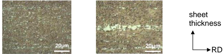
Fig. 2: Light optical micrographs of the TRIP steel along rolling direction, LePera etching. Left: third-thickness microstructure, right: mid-thickness microstructure. Hard phases (austenite + martensite) in white, ferrite in brown.
