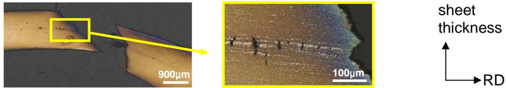
**Fig. 7:** Broken stretch bent specimen and damage at the central segregation area. Optical micrographs, LePera etching
