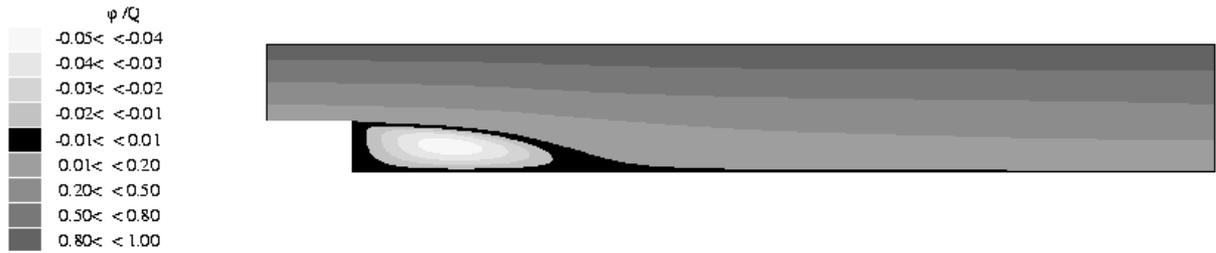
Figure 6: BFS test. Computed stream lines at convergence (iso-values of the stream function  $\varphi$  normalized with the flow rate  $Q$ ).
