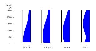
Fig. 4. Liquid mass hold-up profiles at different time instants. At t = 4.5 h, a "slug" is present in the middle of the pipe. It is then expelled over the next 0.2 hours, before a new slug is formed. The velocity of the flow is inhomogeneous in space and time: the slugging cycle comprises phases of acceleration and deceleration.
