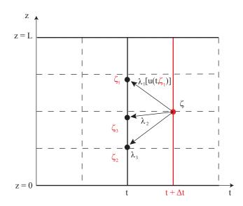
Fig. 2. Solving of the discrete characteristic equations backward in time.
