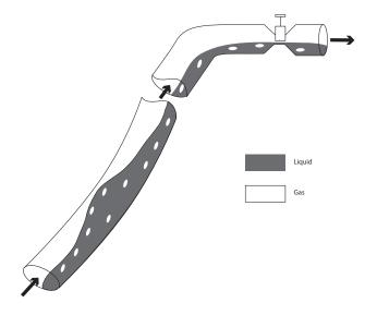
Fig. 1. Inclined pipe transporting oil and gas
