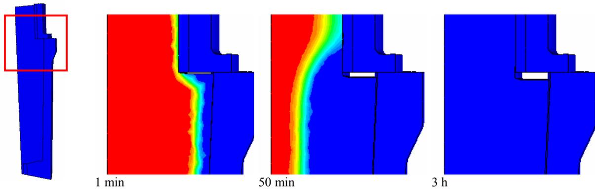
Figure 5. Air gap evolution with liquid fraction distribution.
