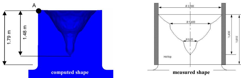
Figure 3. Comparison computation/measurement of pipe shape. Longitudinal section.
