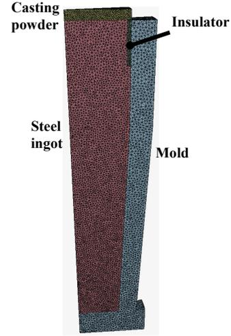
**FIGURE 2.** FEM model of an ingot casting process.
