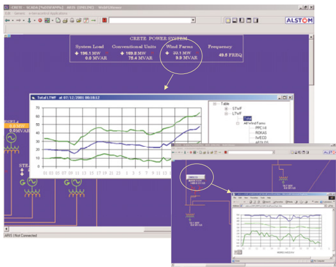
Fig. 9: User interface of an industrial SCADA software integrating the wind power prediction module.
