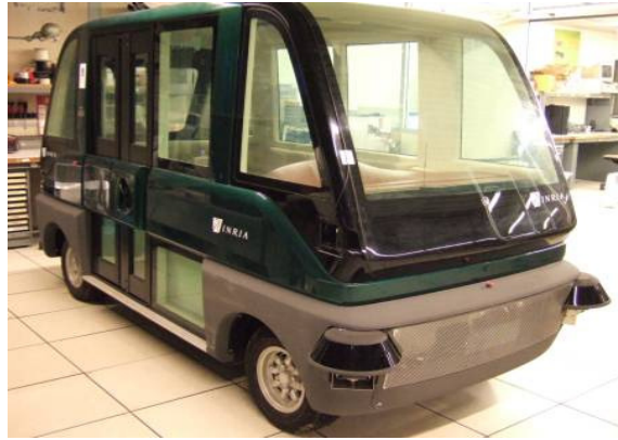
Fig. 5. Dual laser system of AGV.
