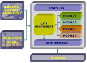
Fig. 1: General architecture of the ANEMOS prediction platform.
