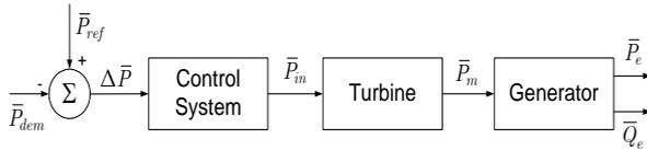
**Figure 1.** Main blocks in microturbine model
