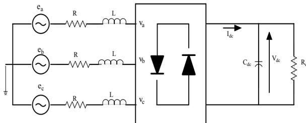
Figure 6. Circuit diagram of three-phase  $VSC$
