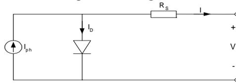
Figure 4. Simplified single-diode model of a solar cell.
