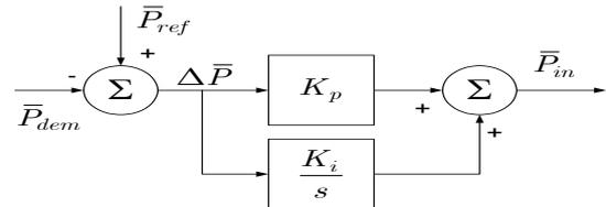
**Figure 2.** Load following control system model.
