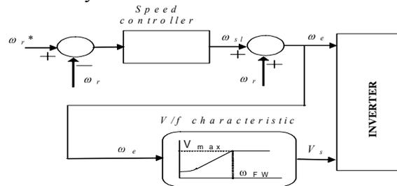
Figure 5. Scalar control system of the generator-side converter.
