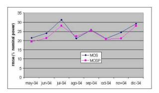
Figure 4: Two methods for downscaling with (MOS) and without (MOSP) intermediate step to wind speed. The plot shows normalised RMSE for forecasted power production at the Alaiz wind farm (ES).
