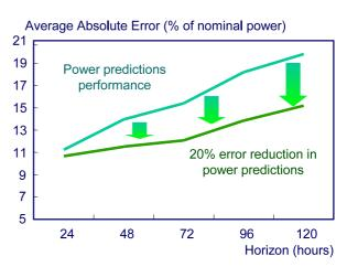
Figure 2: Improvement on average absolute error by using the Kalman filtering
