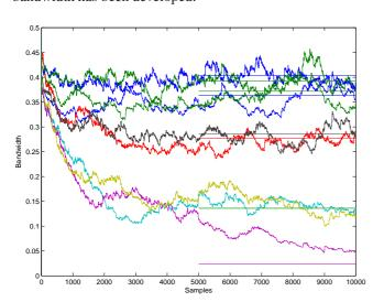
Figure 15: A Gaussian weight function is used to optimise the bandwidth at nine fitting points. Both steepest descent traces and fix bandwidth optimised on the last half of the data are shown.
