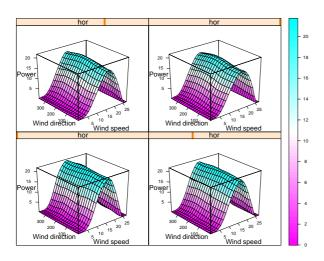
Figure 6: Plots of the estimated power curve for the Klim (DK) wind farm (k = 0, 12, 24 and 36 hours).
