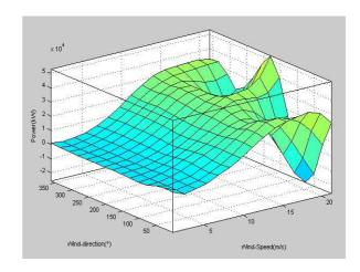
Figure 5: A two-dimensional power curve model
