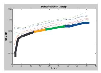
**Figure 11**: Example of individual prediction models (dotted lines) and the expected effect of error reduction by prediction combination in Golagh wind farm. Combination depends on forecast horizon.
