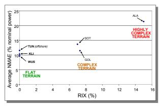
Fig. 2: Average NMAE for 12 hours forecast horizon vs RIX at each test case. Qualitative comparison. TUN is an offshore wind farm in Denmark, KLI is also located in Denmark, WUS in Germany, GOL in Ireland and ALA and SOT in Spain.
