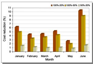
**Fig. 19:** Study on the power system of Crete. Estimation of monthly cost reduction due to improvement in the wind forecasts accuracy. A 6-10% reduction is achieved also in GHG emissions ( $SO_2$ ,  $NO_X$ ,  $CO_2$ ) by the use of an advanced forecasting tool that permits to avoid excessive reserves allocation.
