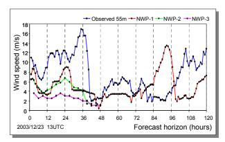
**Fig. 4:** Comparison wind speed measurements (at 55m – bleu line) to NWPs (at 10m) provided by 3 different meteorological models for a complex terrain wind farm site.
