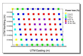
**Fig. 13:** Evaluation of wake effect in a large offshore wind farm. Total wakes power loss is ~10% but individual wake losses are much larger.
