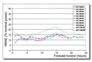
**Fig. 3:** Comparison of the performance of 11 prediction models on the Alaiz wind farm in Spain (very complex terrain). The NMAE is given as a function of the prediction horizon which here is 24 hours ahead.
