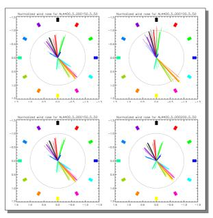
Fig. 5: The wind speed enhancement and turning effect of the topography are dependent on the wind speed, profile and stability configurations. These effects are displayed in the above diagrams showing the mesoscale effect on the geostrophic wind forcings. Details are reported in [39].
