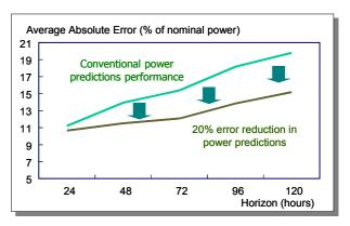
**Fig. 8:** Improvement on the performance of power predictions by using the Kalman approach to filter NWPs.
