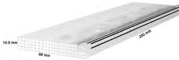
Figure 13: Modelled geometry with the three weld lines indicated by the bold black lines. Please note that three heat sources were required for modelling of the experimental single pass welding. In all the cases the fusion plane is treated as a symmetry plane. The figures show the grid density after the simulation is finished.
