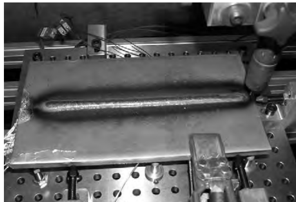
Figure 6: Instrumented test samples align on the bench after the welding.
