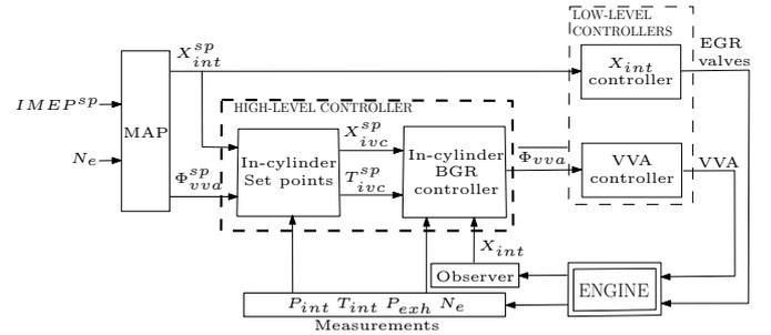
Fig. 5. Control scheme. The cylinder set points  $X_{ivc}^{sp}$  and  $T_{ivc}^{sp}$  are given in Section 4.1. The high-level controller coordinates the low-level controllers using control law presented in Section 4.2 to determine VVA actuator trajectory  $\overline{\Phi_{vva}}$ .
