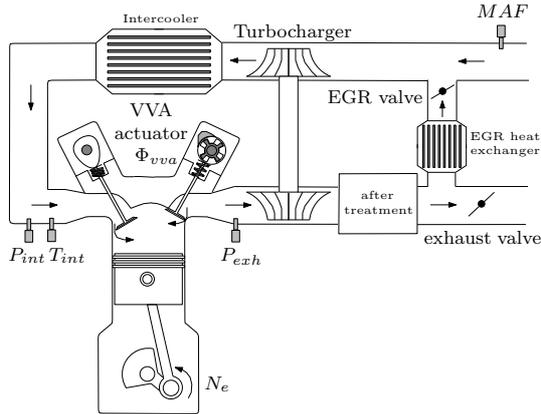
Fig. 1. Schematic illustration of a turbocharged, VVA-equipped Diesel engine. The intake manifold pressure and temperature  $P_{int}$  and  $T_{int}$ , the exhaust manifold pressure  $P_{exh}$  and the mass air flow at the intake  $MAF$  are measured by sensors.  $\Phi_{vva}$  is the position of the VVA actuator.
