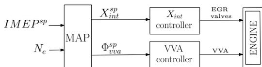
Fig. 2. Classical control strategy.  $IMEP^{sp}$  and  $N_e$  refer to the driver torque demand and the engine speed, respectively. Look-up tables determine set points for the intake manifold BGR and VVA actuator position,  $X_{int}^{sp}$  and  $\Phi_{vva}^{sp}$ .
