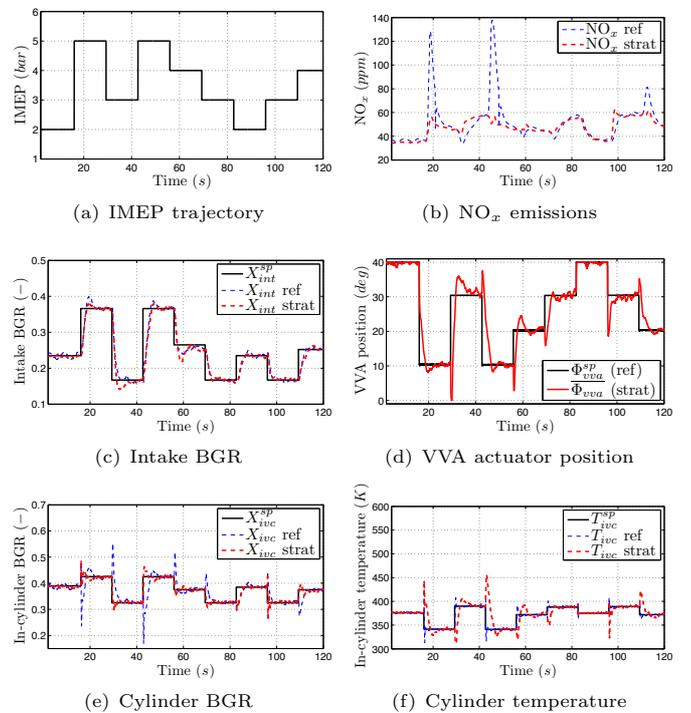
Fig. 7. Test-bench results for a four-cylinder Diesel engine for step torque demand at constant speed of 1000 *rpm* with and without the proposed control strategy. The controller succeeds in tracking the cylinder BGR set point. Consequently, the  $\text{NO}_x$  emissions peaks are reduced.
