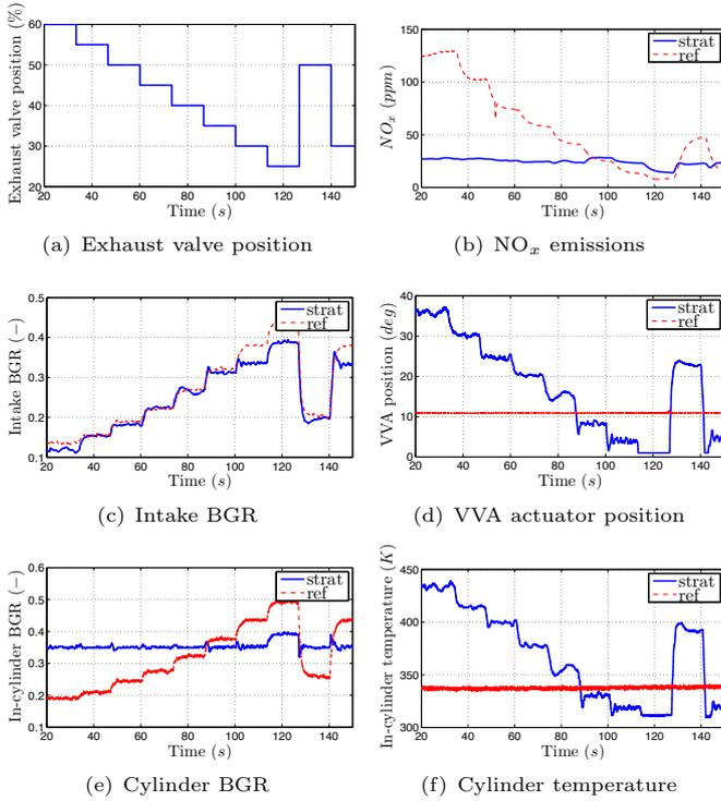
Fig. 6. Test-bench results for a four-cylinder Diesel engine for exhaust valve position variation at constant speed of 1500 *rpm* with and without the proposed control strategy. The controller succeeds in keeping constant the cylinder BGR, and consequently the  $\text{NO}_x$  emissions.
