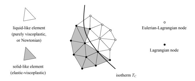
Fig. 3. Lagrangian and Eulerian-Lagrangian nodes, as determined by their belonging to solid-like and liquid-like finite elements. Schematic in two dimensions.
