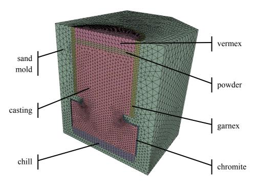
Fig. 6. Finite element mesh of the casting and the six different subdomains of the mould.
