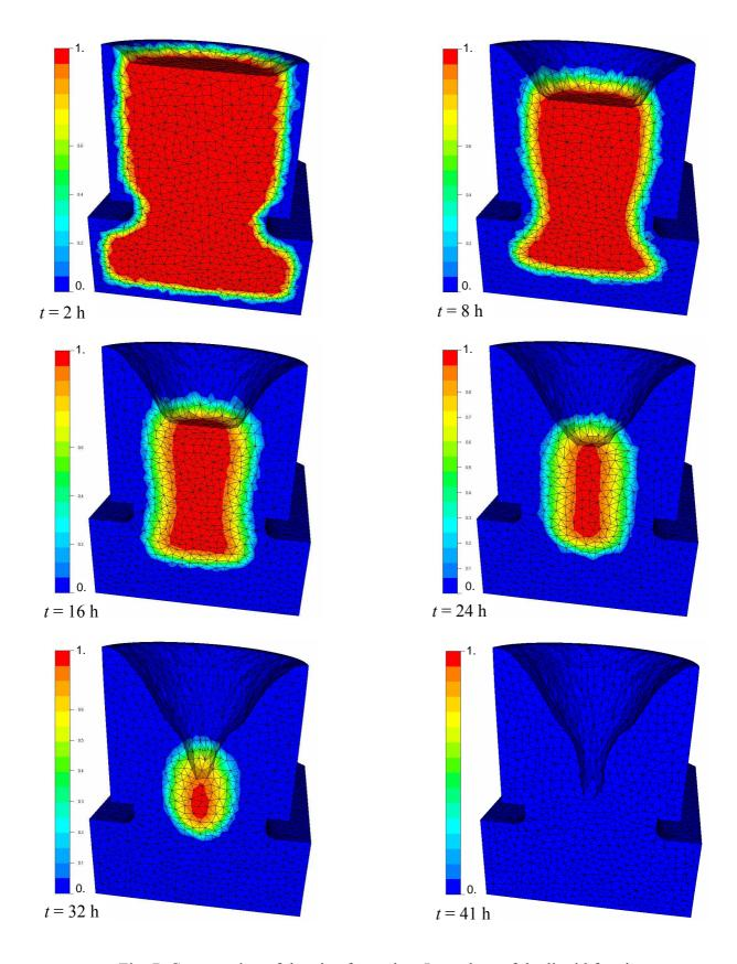
Fig. 7. Computation of the pipe formation. Iso-values of the liquid fraction.
