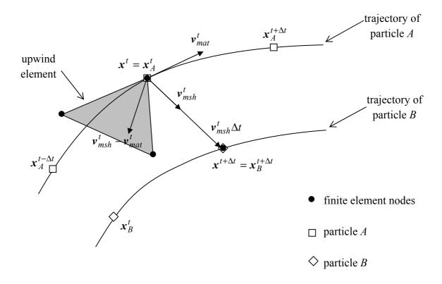
Fig. 2. ALE formulation: schematic in two dimensions. Updating of the location of a finite element node and subsequent identification of the upwind element. The materialization of the trajectory of two material particles A and B helps in the interpretation of equation (30).
