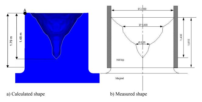
Fig. 8. Comparison of calculated (left) and measured (right) shapes of the pipe. The section plane is the longitudinal mid plane of the part.
