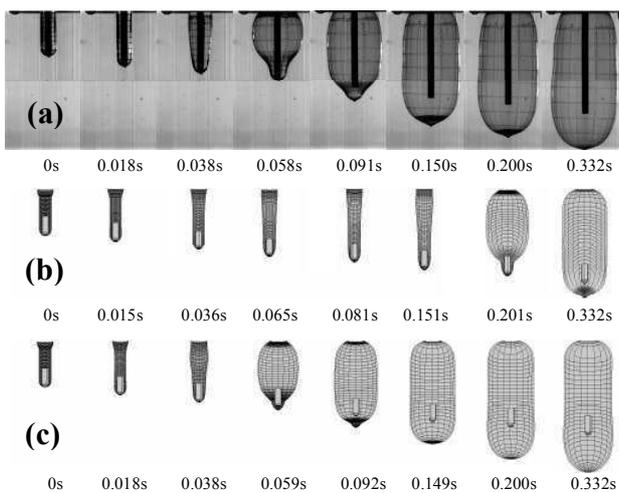
Fig. 7: Preform shape evolution. Experiment (a) vs. simulation via direct pressure (b) and mass flow rate inputs(c).
