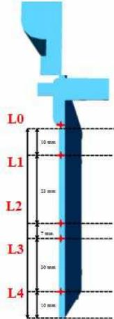
Fig. 4: Positions of samples taken for fibre orientation distribution
