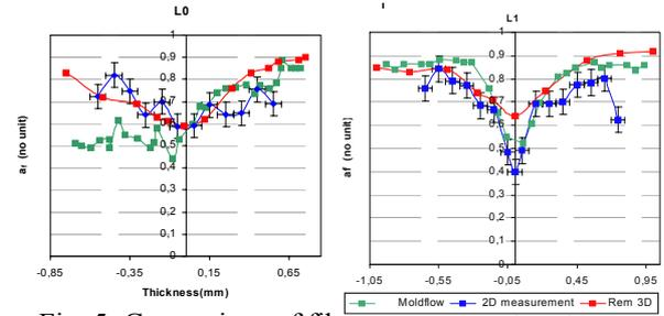
Fig. 5: Comparison of fibre orientation distribution
