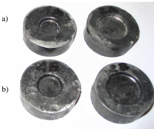
Fig. 6. Closed-die forged preforms: a-Fe-40at% Al, b- Fe-30at% Al
