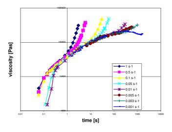
Fig. 2. Transient extensional viscosity for different strain rates at 180 °C.
