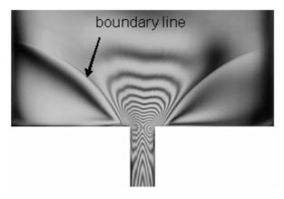
Fig. 5. Birefringence picture at T =  $180 \text{ }^{\circ}\text{C}$  and m = 0.3 g/s.
