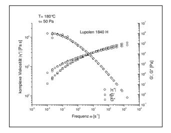
Fig. 1. Master curve at  $180^{\circ}C$  of the complex viscosity and modulus of the material.
