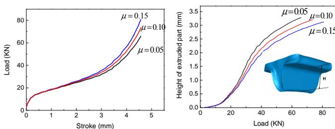
(a) Load (b) Height of extrusion part
