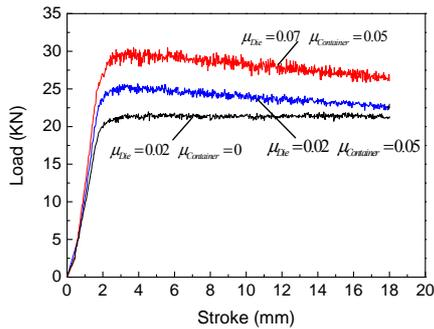
Fig. 3 Effect of friction coefficients of die and container on the extrusion loading curve
