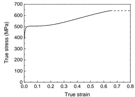
Fig. 1 The strain/stress curve of AISI 1010 by uniaxial compression test (drawn bar with 7.15 mm diameter)
