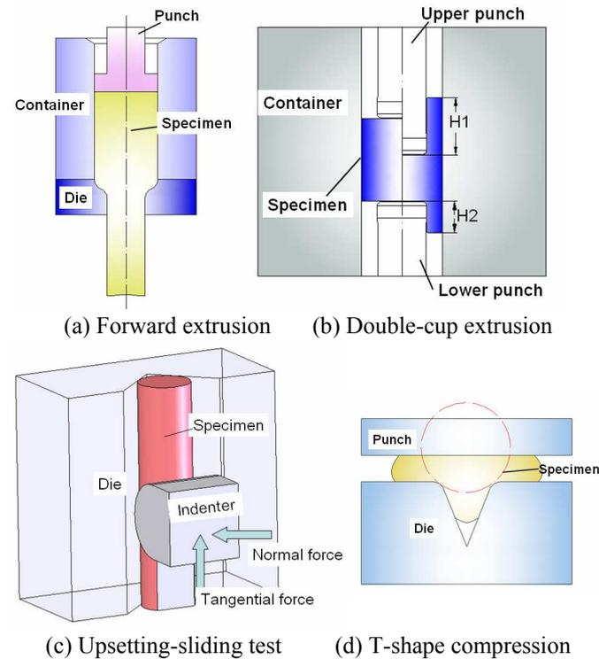
Fig. 1 Friction tests for cold forging
