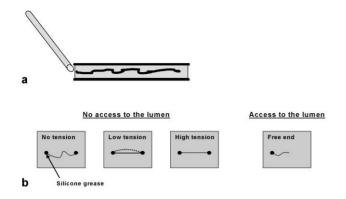
**Figure 1.** Experimental protocol and assembly for studying swelling and dissolution behavior of cellulose fibres in NMMO-water at 90°C. (a), The solvent is injected by capillarity between the two glass plates. (b), Four configurations of experiments: (i) no tension, (ii) under low tension (the fibre loosely attached reaches a low tension state due to the contraction during swelling), (iii) under higher tension, and (iv) free end with an access to the lumen in the case of cotton hairs.
