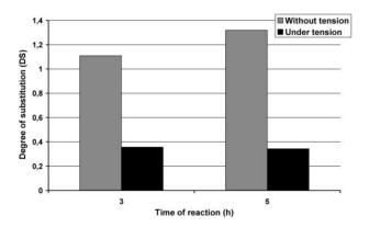
Figure 7. Evolution of the DS with and without tension versus the time of reaction.
