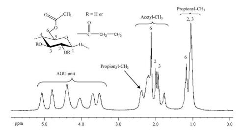
**Figure 6.** <sup>1</sup>H-NMR spectra of the perpropionylated samples without tension, solvent is deuterated chloroform (CDCl<sub>3</sub>).
