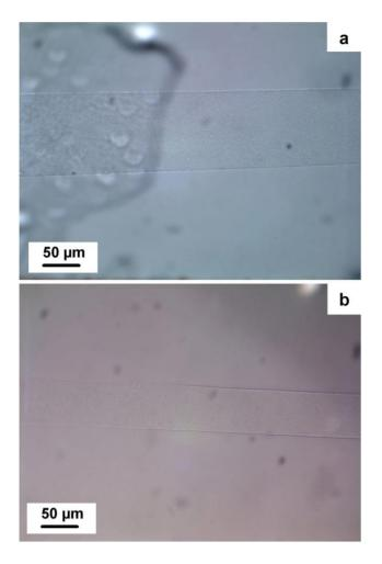
**Figure 4.** NMMO-water: swollen Tencel fibres under varied conditions of tension. (a) Very large homogeneous swelling (ratio 9.5) right before the dissolution, no tension was applied to the fibre. (b), Lower homogeneous swelling (ratio 5.2), the fibre is under low tension.
