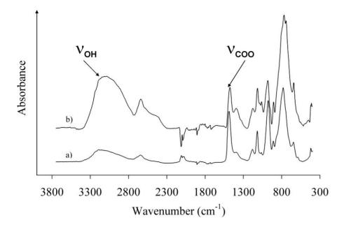
Figure 5. Example of FTIR spectra of acetylated Alceru fibres: a) without tension; b) with tension.
