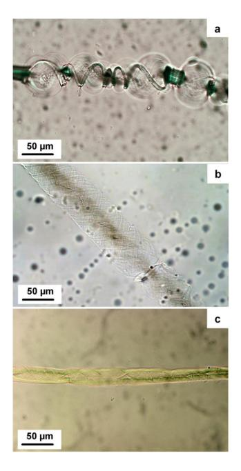
**Figure 3.** NMMO-water: swollen cotton hairs under varied conditions of tension. (a), Swelling by ballooning (ratio 5.3) right before the dissolution, no tension was applied to the fibre. (b), Large homogeneous swelling (ratio 4.8) and no dissolution, the fibre is under low tension. (c), Low homogeneous swelling (ratio 2) and no dissolution, a higher tension was applied to the fibre.
