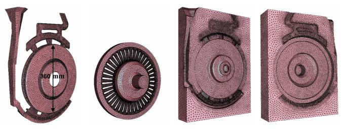
Figure 5. Finite element meshes of the different domains: part, core, and two half molds.
