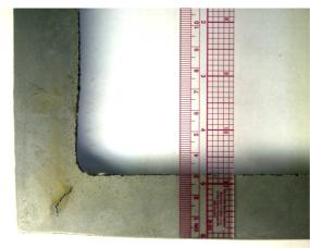
Figure 15. Off-corner internal crack in break-out shell from a 175 mm square bloom.
