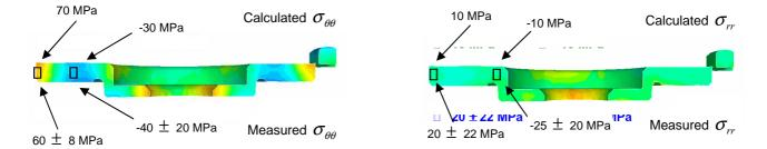
Figure 8. Residual hoop stresses (left) and radial stresses (right) in a radial section on as-cast plain discs made of grey iron. Top line: calculated values; bottom line: measured values.
