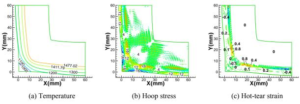
Figure 14. Distorted contours at 200 mm below mold exit.
