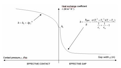
Figure 1. Modeling of the local heat transfer coefficient in the gap and effective contact situations.
