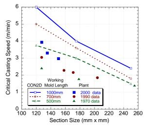
Figure 16. Comparison of critical casting speeds, based on hot-tearing criterion, and typical plant practice.<sup>[87]</sup>
