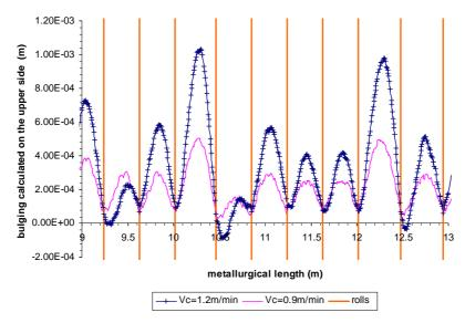
Figure 10. Slab bulging calculated at two different casting speeds: 0.9 m/min and 1.2 m/min. The slab bulging increases with the casting speed.<sup>[67]</sup>
