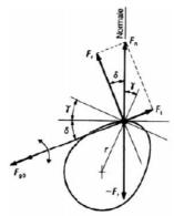
Figure 5: Forces applied on disc cam and follower with a roller [6].
