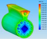
Figure 9: Deformation of the compressor rotor.
