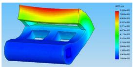
Figure 10: Deformation of the compressor thrust.
