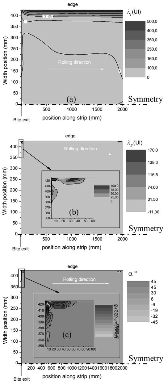
**Figure 3:** Flatness defect prediction. a : first principal buckling strain  $\lambda_I$ , b : second principal buckling strain  $\lambda_{II}$ , c : angle  $\alpha$  defining the eigendirections of the buckling strain  $\lambda$ .
