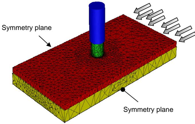
Figure 1: Global view of the finite element model.
