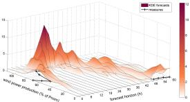
Figure 2. Example of probability density function forecasts.
