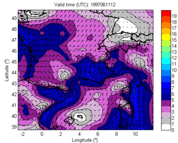
Figure 10: 10 m wind speed field simulated by RAMS at a 25 km horizontal resolution on the 11<sup>th</sup> June 1997 at 12Z. The wind direction is given by arrows and the wind speed (m s<sup>-1</sup>) by colours. This field participates in building the event 10 (Fig. 6).
