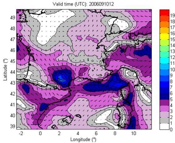
Figure 12: 10 m wind speed field simulated by RAMS at a 25 km horizontal resolution on the 10<sup>th</sup> September 2006 at 12Z. The wind direction is given by arrows and the wind speed (m s<sup>-1</sup>) by colours. This field participates in building the event 14 (Fig. 8).
