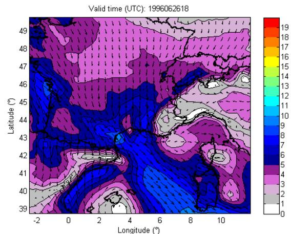
Figure 11: 10 m wind speed field simulated by RAMS at a 25 km horizontal resolution on the 26<sup>th</sup> June 1996 at 18Z. The wind direction is given by arrows and the wind speed (m s<sup>-1</sup>) by colours. This field participates in building the event 12 (Fig. 7).
