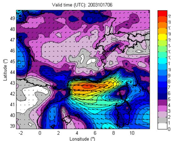
Figure 9: 10 m wind speed field simulated by RAMS at a 25 km horizontal resolution on the 17<sup>th</sup> October 2003 at 06Z. The wind direction is given by arrows and the wind speed (m s<sup>-1</sup>) by colours. This field participates in building the event 3 (Fig. 5).
