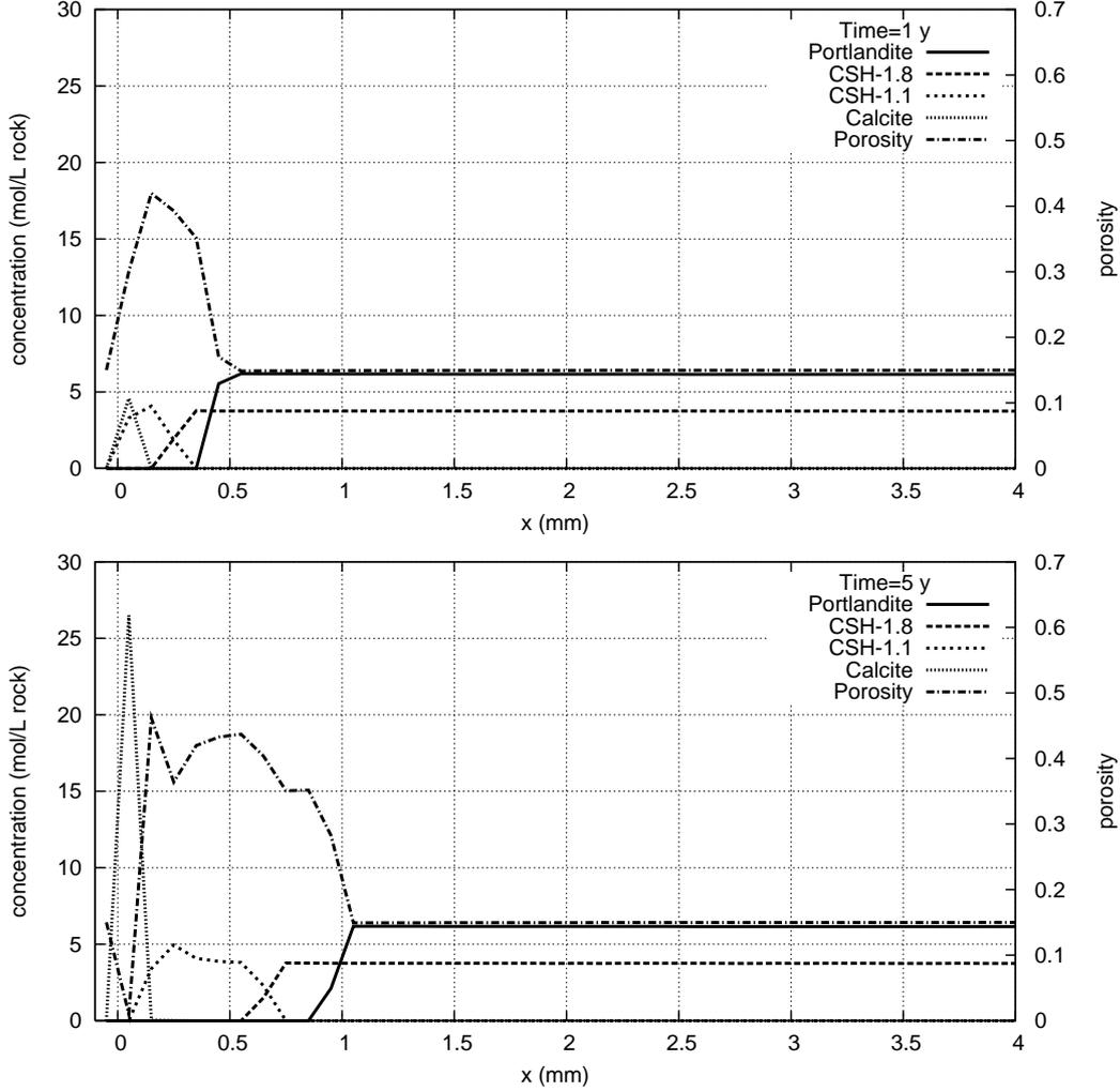
Fig. 7. Profiles of main mineral phases and porosity during degradation and carbonation of a cement. A sharp drop in the porosity is observed at the cement-fluid interface.
