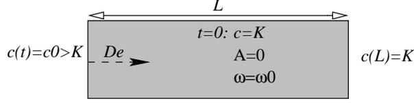
Fig. 1. Schematic representation of the second analytical problem.
