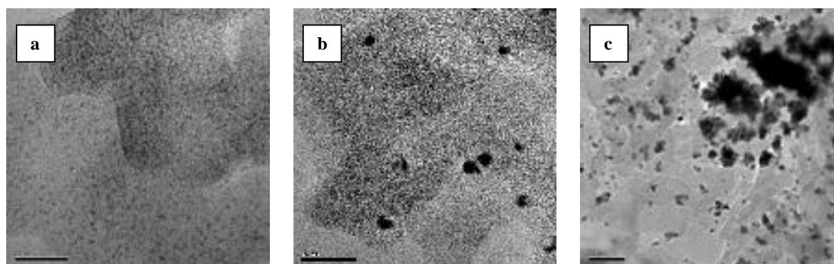
**Figure 1:** TEM images showing Pt adsorption on CA after reduction with (a)  $\text{H}_2$ , scale bar 20 nm (b)  $\text{NaBH}_4$  after filtration, scale bar 50 nm and (c)  $\text{NaBH}_4$  before filtration, scale bar 50 nm.
