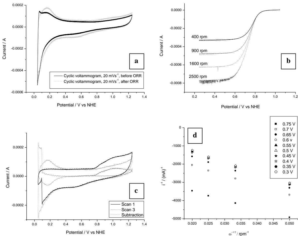
**Figure 3** : Voltamperograms for (a) adsorption-desorption of hydrogen, (b) oxygen reduction reaction, (c) CO stripping before the oxygen reduction reaction and (d) Koutecky-Levich graphs for sample I, Pt/CA reduced under  $H_2$  at  $300\text{ }^\circ\text{C}$ . Results obtained using a rotating disk electrode.
