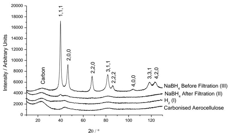
**Figure 2** : XRD patterns showing Pt adsorption on CA after reduction with H<sub>2</sub> and with NaBH<sub>4</sub> either before or after filtration. The pattern generated from the CA support is also shown.
