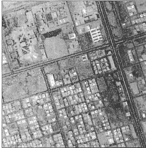
Figure 2. Extract of the panchromatic band of the KVR-1000 Russian sensor at 2 m of spatial resolution on Jeddah (Saudi Arabia).
