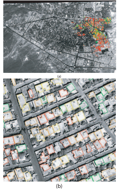
Fig. 1. QuickBird reference image (before the earthquake) of Bam. The buildings footprint of the corresponding reference database is overlaid. (a) : entire scene; (b) : image extract. Colour legend of the database: Green = damage grade 0; Yellow = damage grade 3; Orange = damage grade 4; Red = damage grade 5. Images: copyright DigitalGlobe 2003, 2004.
