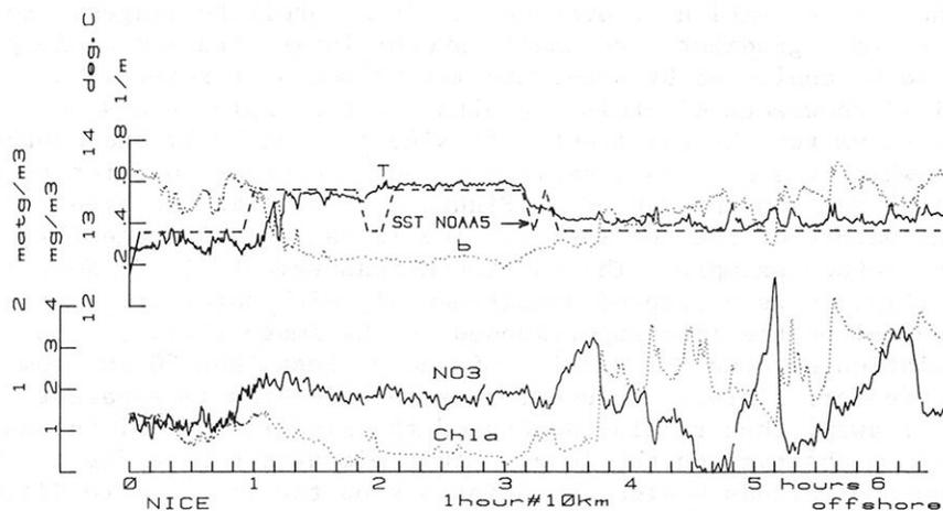
Fig. 3: Ship data of 7 March 1978 for pigments (Chla,  $\text{mg.m}^{-3}$ ), nitrate ( $\text{NO}_3$ ,  $\text{matg.m}^{-3}$ ), temperature (T, deg. C) and total scattering coefficient (b,  $\text{m}^{-1}$ ) at the depth of 3 m, along the longer track on Fig. 2.
